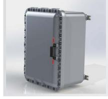
For EJB-6/6B and EJB-7/7B junction boxes, the opening and closing of the cover is facilitated by the presence of an even more sturdy handle, able to offer a greater safety of use for the operator. It is made of stainless steel AISI 316L, which, after a blasting process, is coated with a matt black powder (RAL 9005) coating that ensures pleasing aesthetics and a high resistance to physical impact and corrosion in saline environments.
